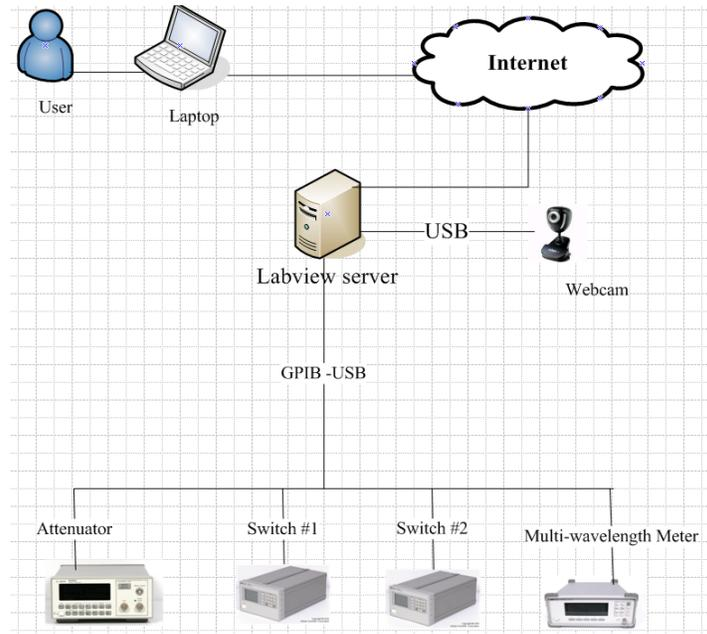
Figure 1: LabVIEW-based remote optical communications laboratory.
