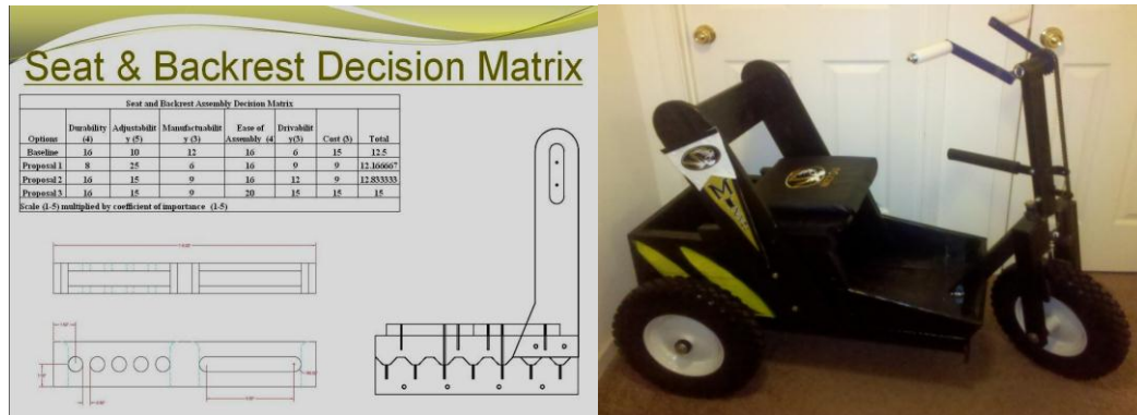
Fig.1 Seat & backrest decision matrix and PET prototype (MU)
