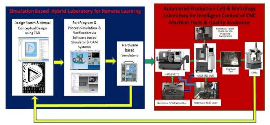
Figure 1. Overall architecture of proposed project.
