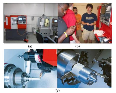
**Figure 2** (a) EMCO CNC TC and Haas VMC located at Engineering Technology Mechanical Laboratories (b) ETStudents are being trained on EMCO CNC TC with Fanuc control. (c) Various test parts machined using EMCO TC.
