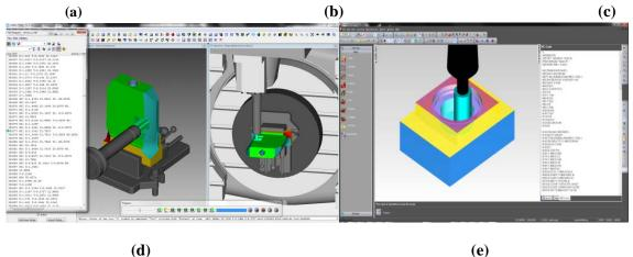
**Figure 4.** (a) HAAS dual system control simulator hardware. (b) Swansoft CNC simulation software showing machine control panel simulation for HAAS control. (c) Swansoft CNC simulation software showing machine control panel simulation on a tablet pc for Fanuc control. (d) VERICUT CNC machining and program verification software (e) FeatureCAM part program generation.
