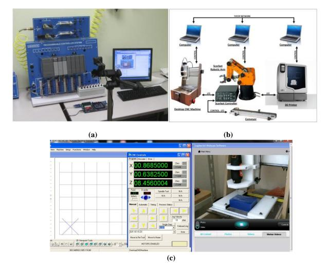
**Figure 6.** (a) Workstation used for online laboratory exercises at Drexel University. The board on the table is used in microcontroller experiments. (b) Future machine development remote Work Cell Example at Drexel University. (c) Remote online access to CNC mill located at BCC campus.
