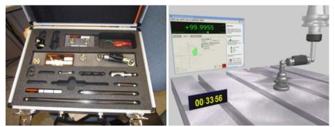
**Figure 1** Renishaw QC20-W (Wireless) Ballbar System in its protective carrying case (left) and Ballbar application simulation software (right)
