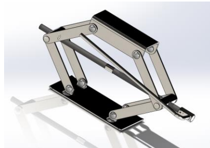
Figure 1 the isometric view of the scissor jack model
