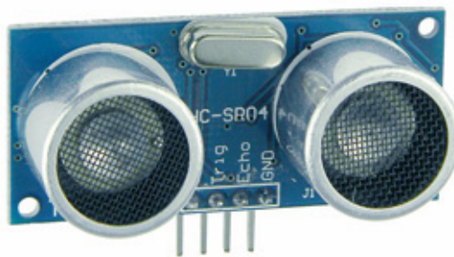
Figure 3. Rangefinder module. The four pins at the bottom are, from left to right, Power (5 V), Trigger, Echo, and Ground.
