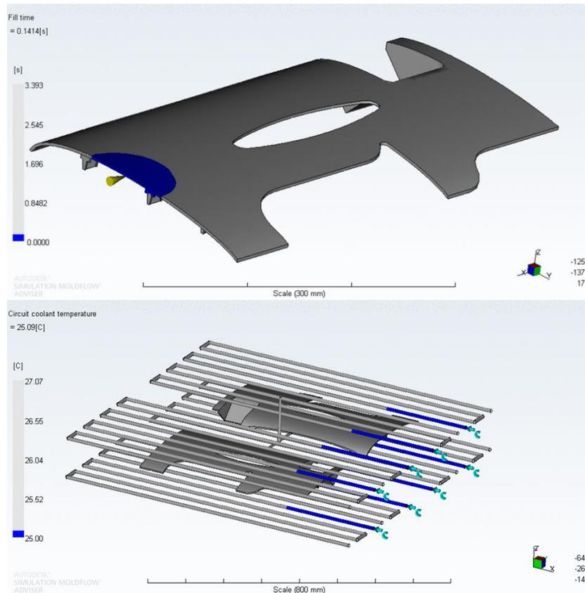
**Figure 7. Moldflow Analysis (a) Fill time (b) Circuit Coolant Temperature – Preparation in progress for the next semester**
