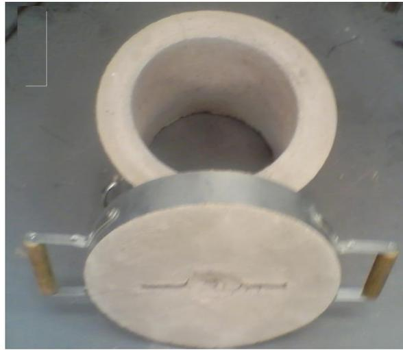
Figure 4. Crucible components for Melting Aluminum
