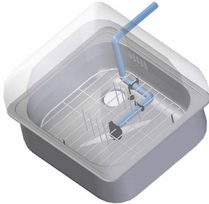
Figure 3. An automatic dishwasher for use in regular sinks. The pipe is manually connected to the tap and draws energy from the water pressure in the existing water pipes.
