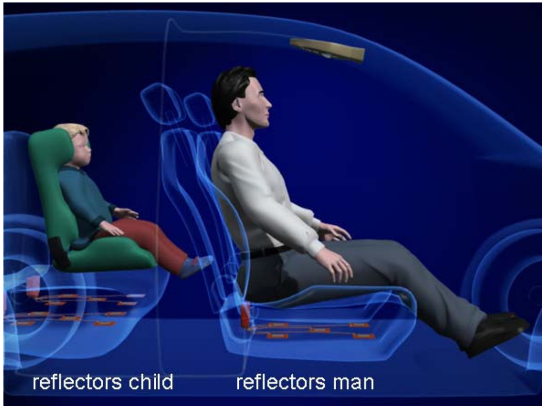
Figure 5. An illustration of the adaptive airbag system as developed in the capstone project.
