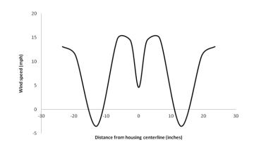
Figure 6. Wind speeds along centerline of fans at 2 inches above housing (approximately 5.5 inches above top plane of rotating fan blade).
