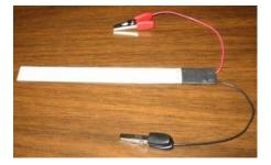
Device size (mm):  $130 \times 10 \times 1$ Active elements: AFCB Mode:  $d_{33}$ Full scale voltage range (V):  $\pm 400$ Full scale power range (mW):  $\pm 120$
