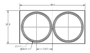
Figure 5. Fan housing dimensions (top view, inches)
