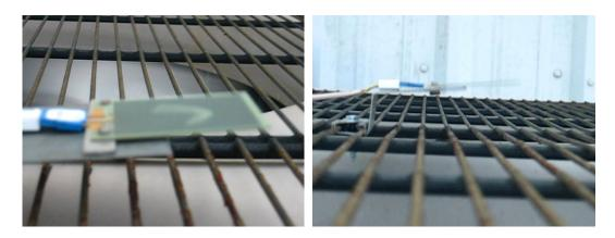
Figure 14. Mide volture piezoelectric device under testing - mounted to exhaust grid
