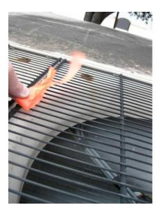
Figure 11. Tape held close to X=0 location. Flow was small and almost horizontal or slight vacuum in this region.
