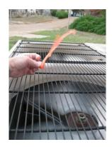
Figure 9. Tape held the in area of maximum airspeed showing angle of flow (partially induced by slight ambient wind, but mostly due to rotational flow).
