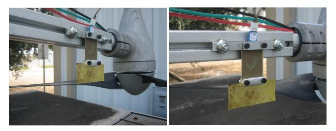
Figure 13. Mide volture piezoelectric device under testing – mounted to wind turbine stand
