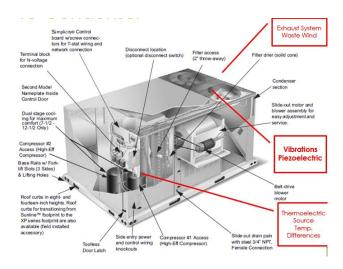
Figure 4. Pictorial of AC condenser unit showing waste energy sources for energy harvesting
