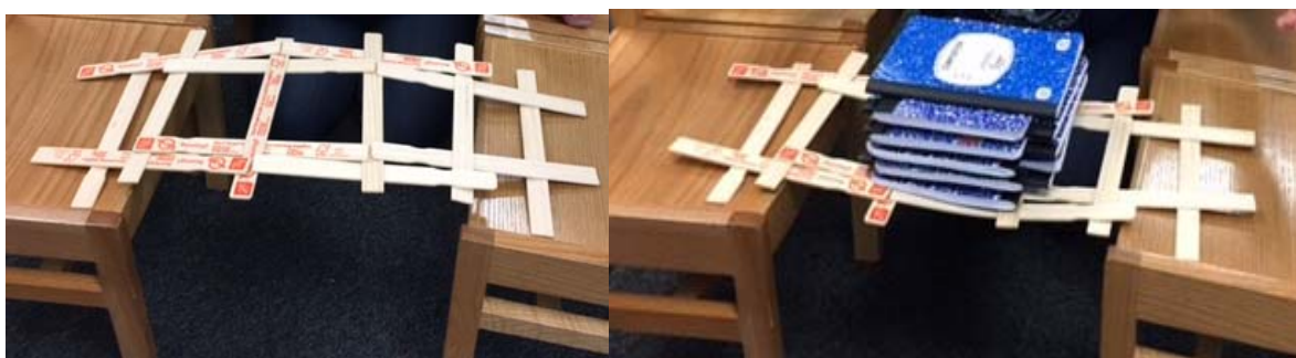
Figure 11-12. Leonardo's Arched Bridge design with paint sticks.
