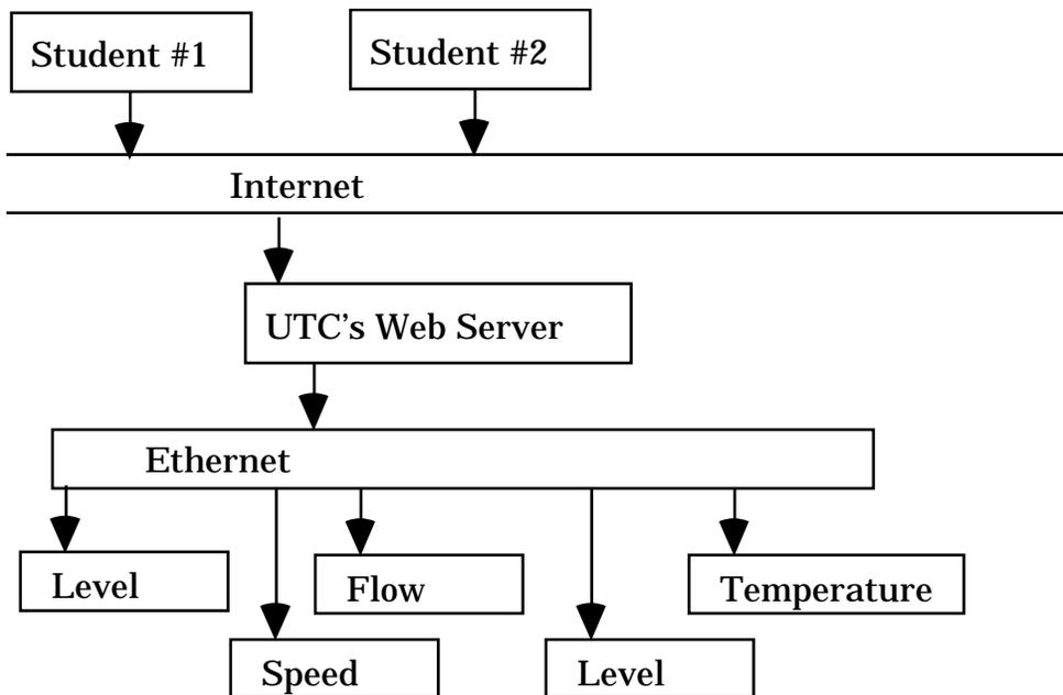
Figure 1: Schematic of communications with lab equipment
