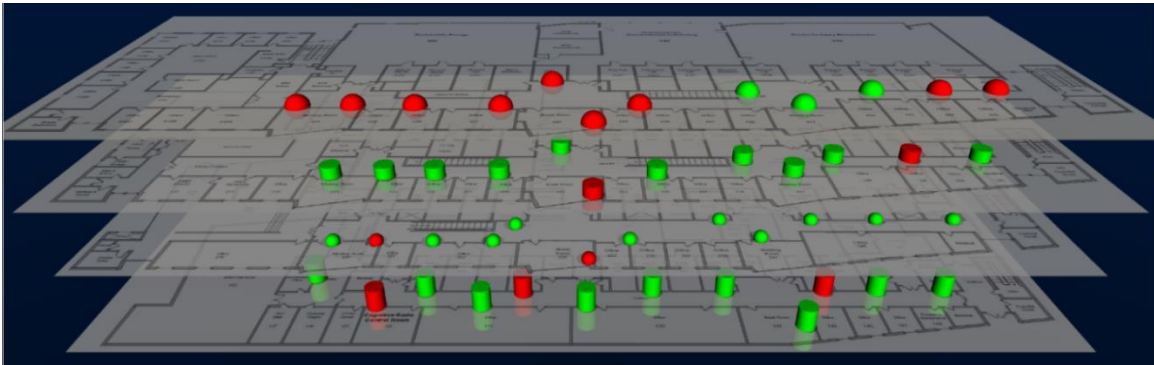
Fig. 2. The CORNET testbed floor plan with the 48 radio front ends as an HTML5 X3DOM data-driven visualization.
