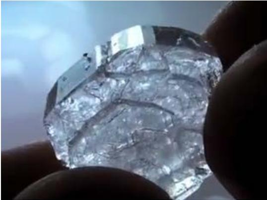
Figure 3. Piezoelectric Rochelle salt crystal made in the lab.
