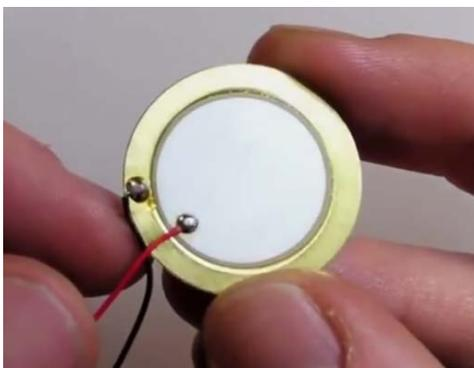
Figure 2. Ceramic Piezoelectric Transducer.
