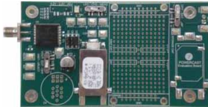
Figure 7- P2110 RF energy harvester evaluation board
