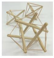
easy to build using rubber bands and wooden dowels. During this session, participants will be introduced to tensegrity and will build basic tensegrity structures that they may keep.
