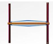
each other. Add one dowel from a different group perpendicular to and in the middle of the original two dowels, so that it looks like an H.
