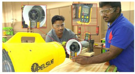
Figure 2: Wind Speed Data collection (students with Civil and Mechanical Engineering backgrounds)
