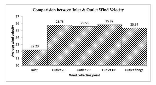
Figure 4: Average Wind Velocity Comparison for various experimental setup
