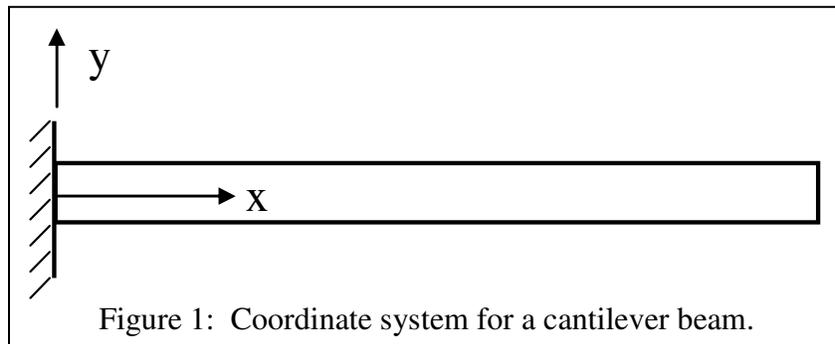
In the present version of the exercise, the problem was simplified by the use of a symmetric cross-section, and since  $I_{yz}$  therefore goes to zero, the bending stress equation simplifies to:
