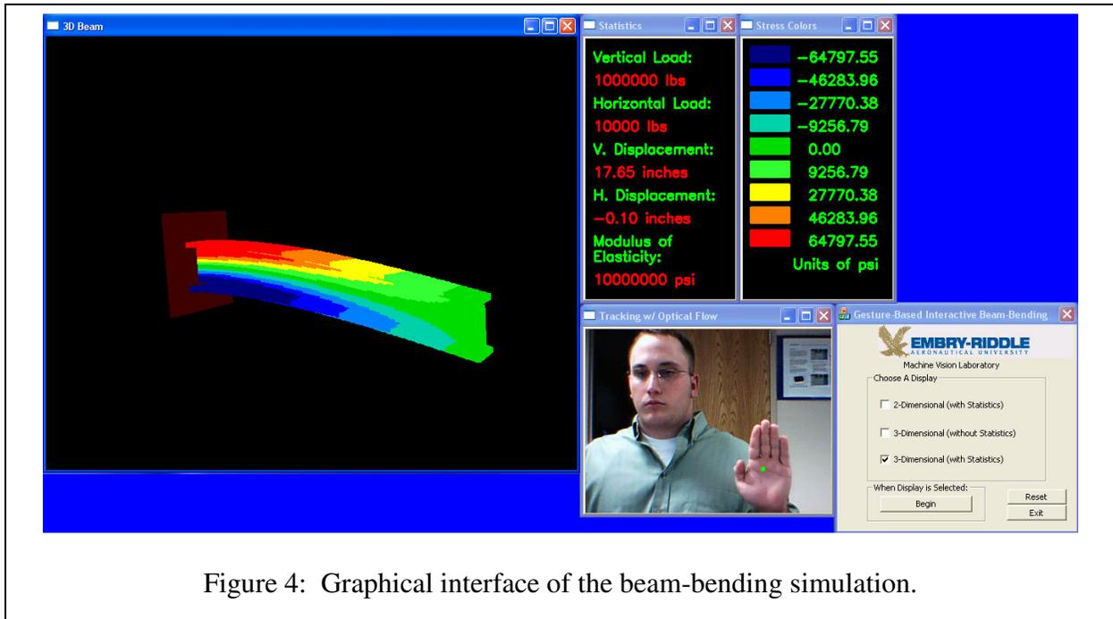
Figure 4: Graphical interface of the beam-bending simulation.
