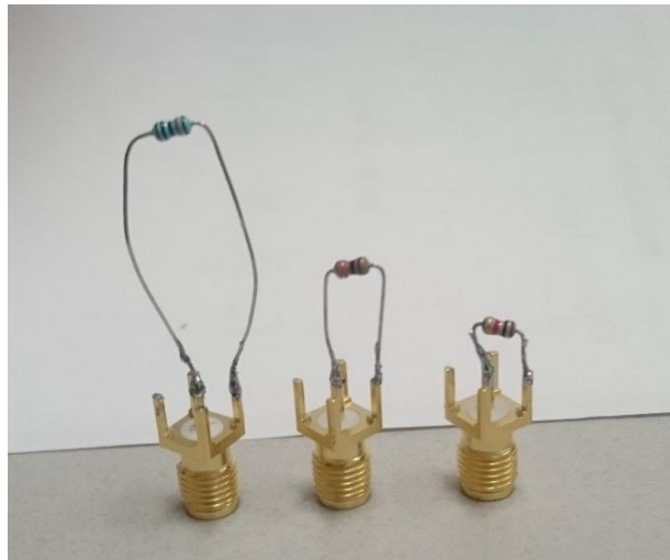
Figure 3 - Example SMA Connector-Resistor Pairs
