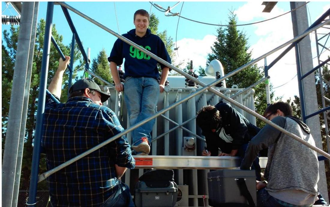
Figure 4. Students Performing an Insulation Resistance Test on a Three-Phase, 2500 kVA Transformer
