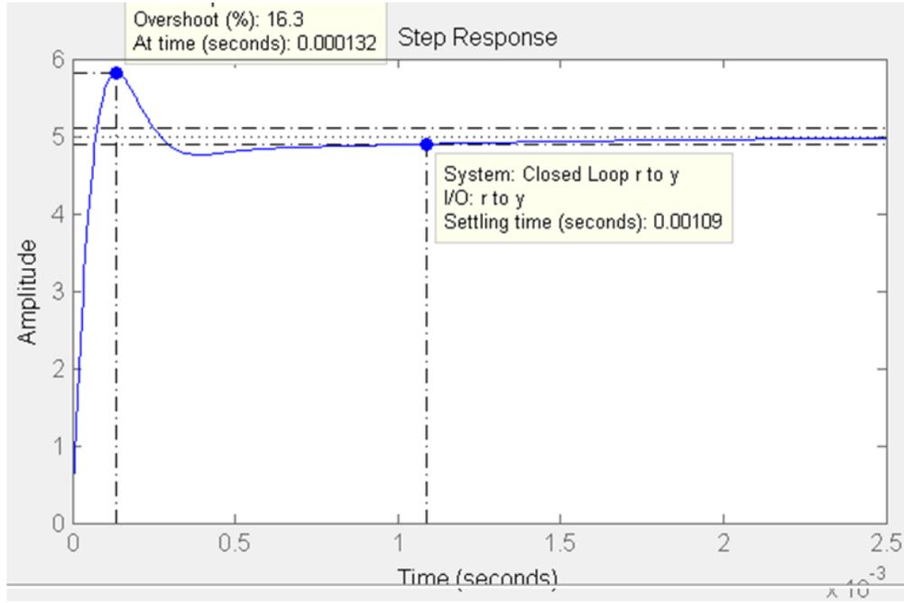
Fig. 8: Unit step response of the buck converter system
