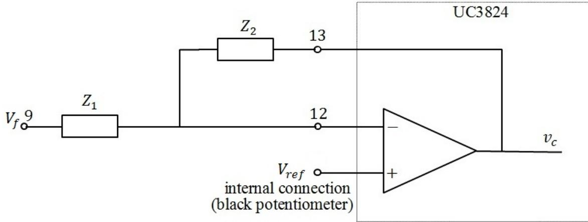
Fig. 9: Hardware implementation of the controller on the power pole board
