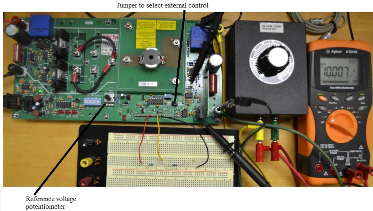
Fig. 10: Experimental setup showing PI controller implementation on the power pole board
