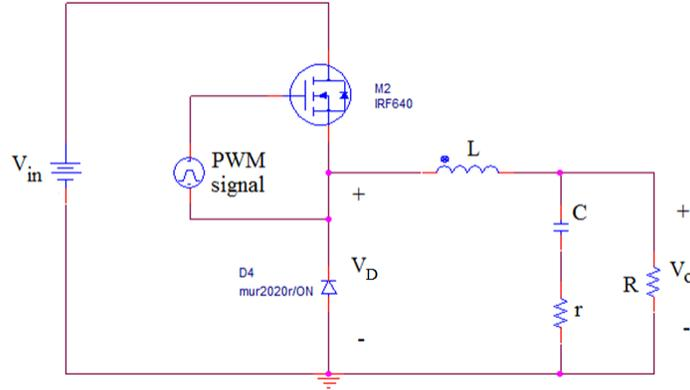
Fig. 4: Buck Converter Schematic
