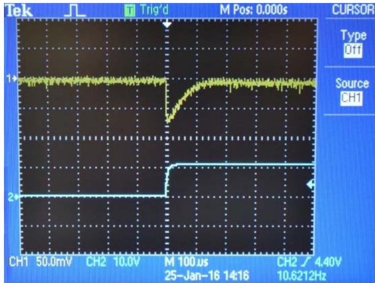
Fig. 11: Output voltage error waveform upon addition of switched load
