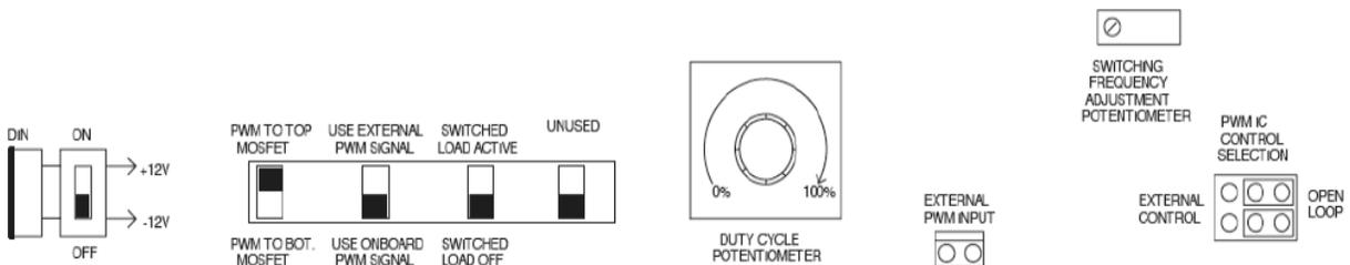
Fig 2: Switches, potentiometers, and jumpers to configure the PPB
