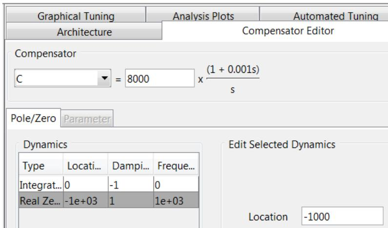
Fig. 6: Compensator editor window showing pole and zero locations and transfer function
