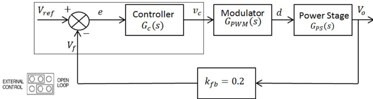
Fig. 3: Block diagram of the buck converter control system
