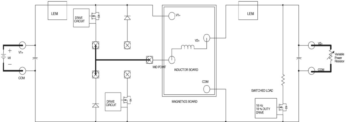
Fig 1: Interconnections to configure the PPB as a buck converter
