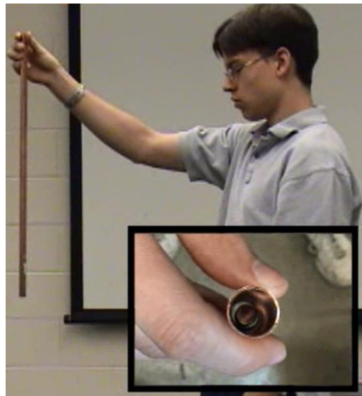
Figure 9. Magnet dropping through a copper tube, an example of a motivating experiment for a writing assignment.
