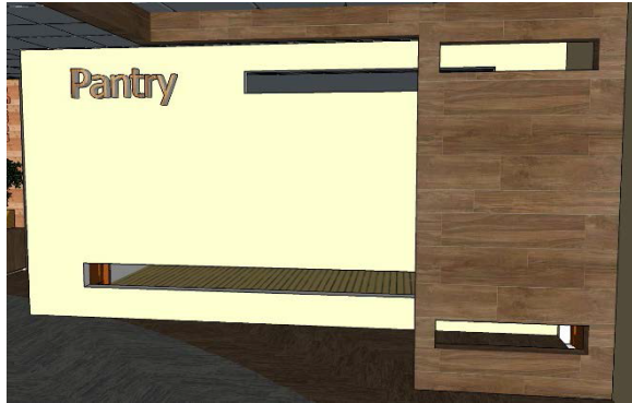
Figure 4. Visibility through the space is permitted with the addition of cutouts in the west wall of the pantry as recommended by Rengel leading to patterns of prospect and mystery . The space is still private and non-visible to patrons of the facility until they proceed into the pantry area.
