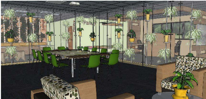
Figure 5. Biophilic pattern number 11, prospect , is shown with floor-to-ceiling glass enclosures, which permit visibility throughout the facility while also keeping the multi-purpose and conference area private.
