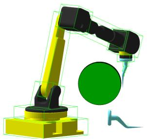
Figure 4: The robot is shown with the part that is grinded on the grinding wheel by rotating using tool frame created.
