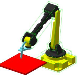
Figure 6. Applying glue on the rectangular sheet in a zigzag manner over the complete area using register and offset instructions.
