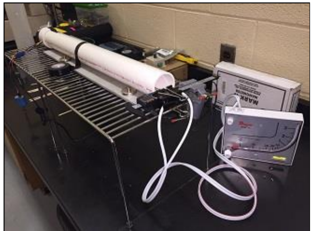
Figure 7: This laboratory-scale velocity profile interrogation experiment (Left) uses HVAC ducting with a diameter too large to allow the flow to develop fully within the length of the apparatus. By contrast, the smaller diameter of the @HOLM™ velocity profile interrogator (Right) enables a measureable fully developed turbulent velocity profile to be formed in less than 1 meter of pipe.
