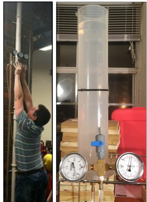
Figure 2: (Left) A full-scale stand pipe is used in conventional fluids labs to demonstrate hydrostatic pressure at depth. (Right) For remote learners, a miniaturized stand pipe has been created with multiple pressure gauges attached to a traveling manifold.
