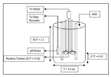
Figure 2. Schematic sketch of the stirred tank.
