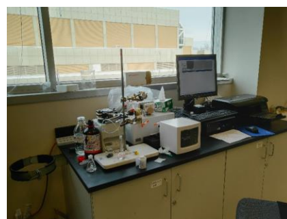
Figure 5: Left and Right are Images of the Peristaltic Pump and FIA set up.
