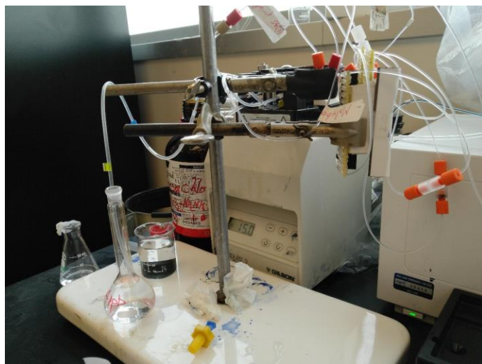
Figure 5: Left and Right are Images of the Peristaltic Pump and FIA set up.
