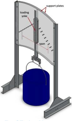
Figure 5. Hanging weight truss tester.
