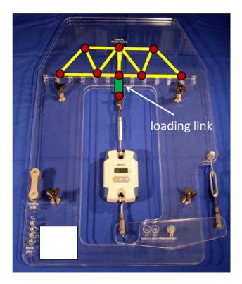
Figure 7. Turnbuckle style tester with the location of the paper truss shown.
