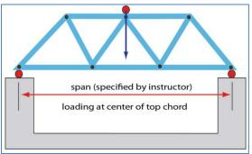
Figure 1. Sample loading configuration for the truss.
