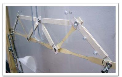
Figure 6. Paper truss loaded in a hanging weight truss tester.
