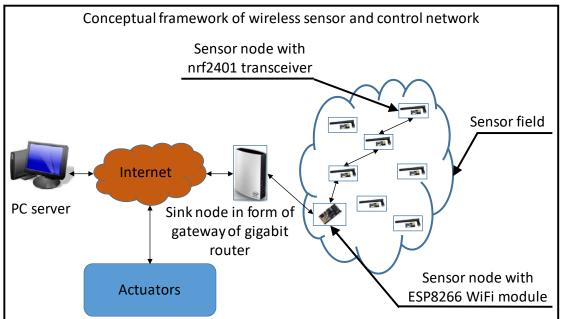
Figure 4: Conceptual framework of wireless sensor and control network
