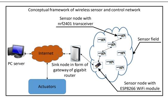
Figure 1: A PC server-based wireless sensor network topology
