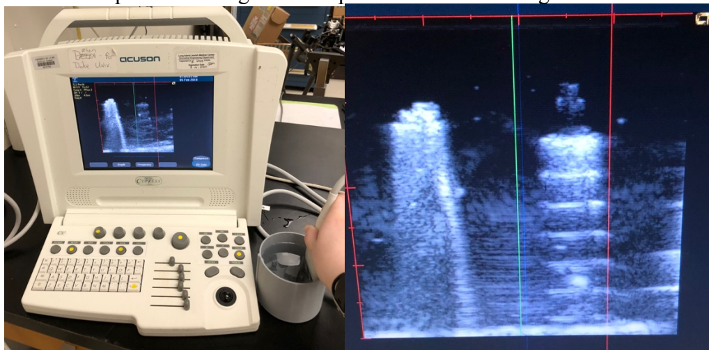
Figure 5: Setup of ultrasound experiment (left) and ultrasound image of the same phantom shown in figure 1 (right)
