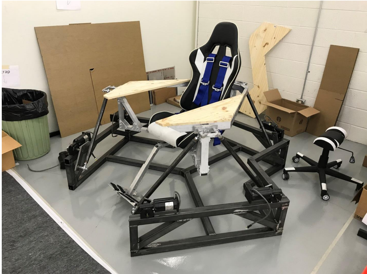
Figure 7: Photograph Showing the Current Status of Stewart Platform Fabrication
