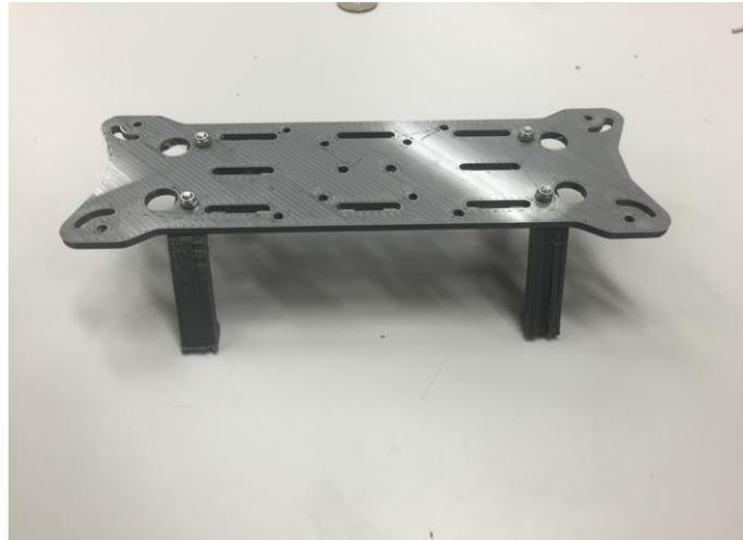
Figure 7: Base Plate with Legs
