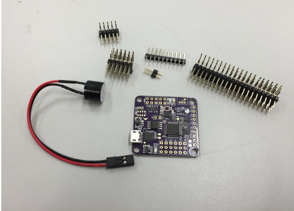
Figure 2: Flight Controller and Piezo Buzzer
