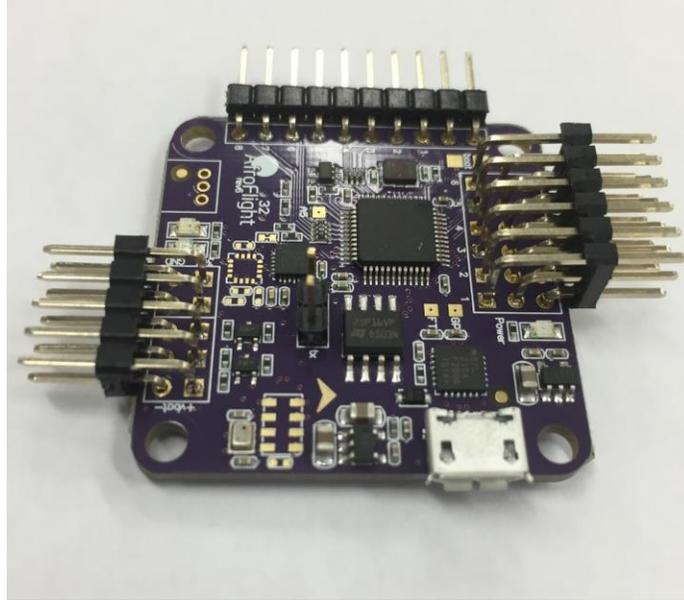
Figure 11: Completed Flight Controller
