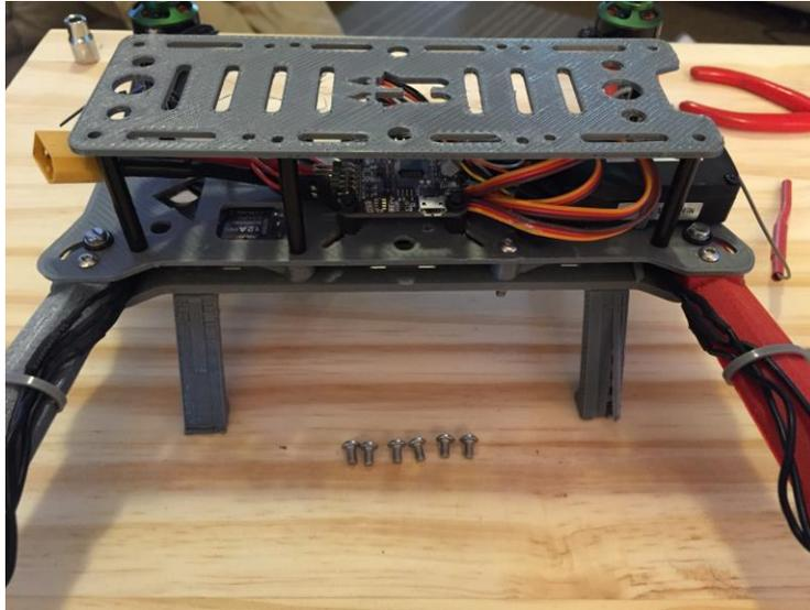
Figure 16: Attaching the Top Plate of the Frame
