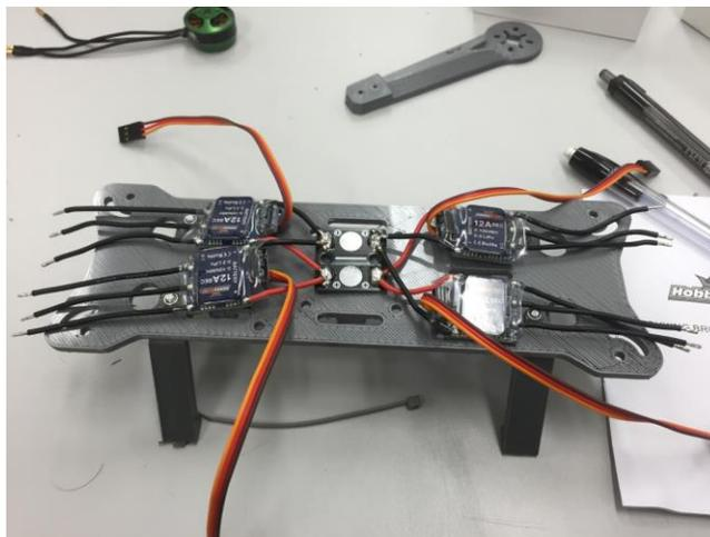
Figure 9: Electronics Attached to Base Plate
