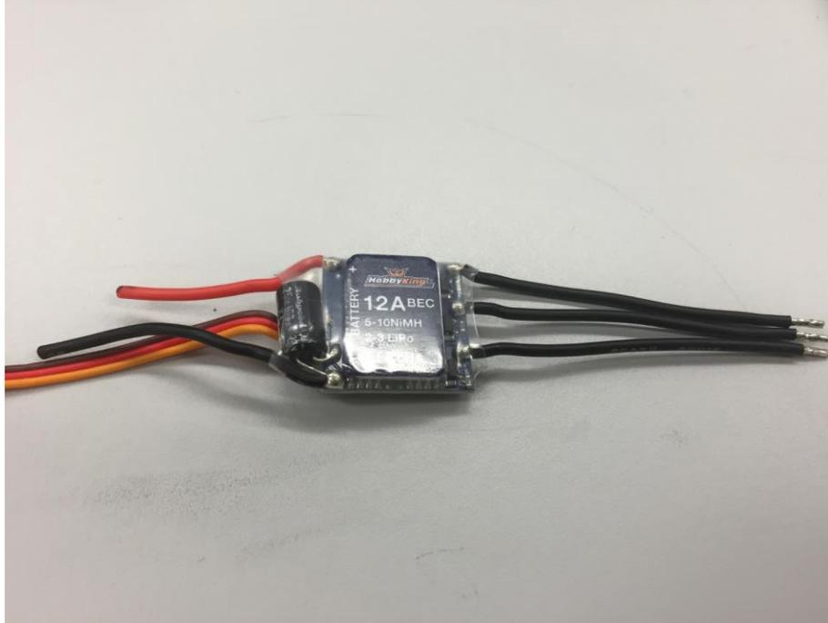
Figure 3: Electronic Speed Controller (ESC)
