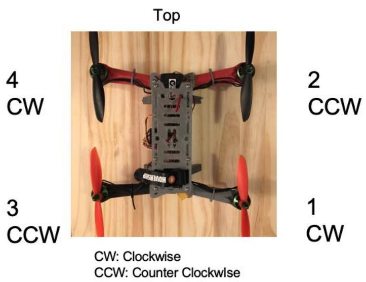
Figure 13: Motor Numbers and Directions
