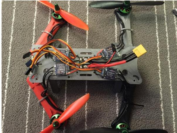
Figure 14: Motors Attached to the Arms
