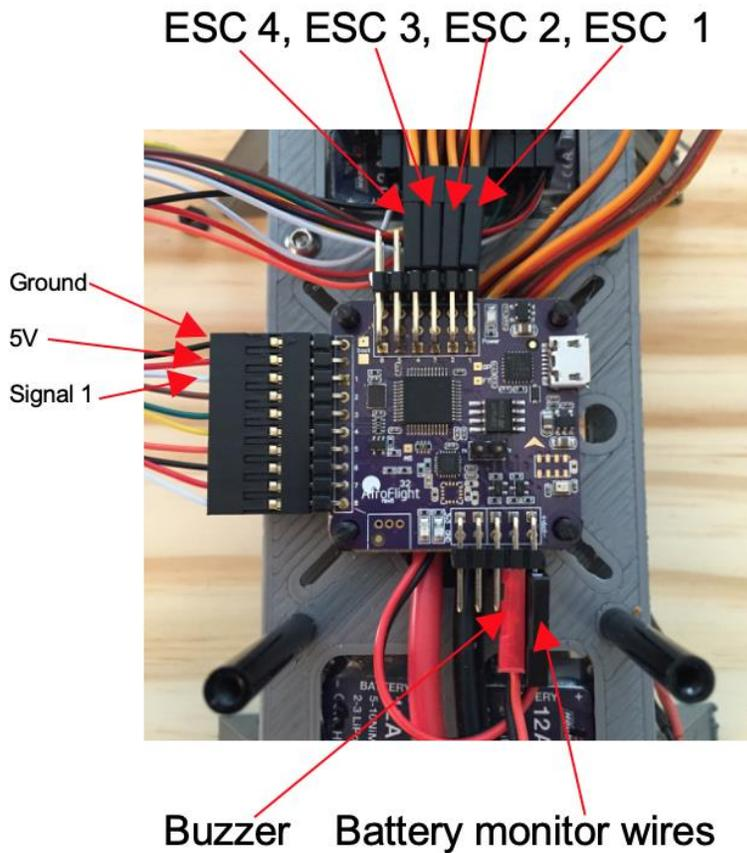
Figure 15: Wire Connections to Flight Controller
