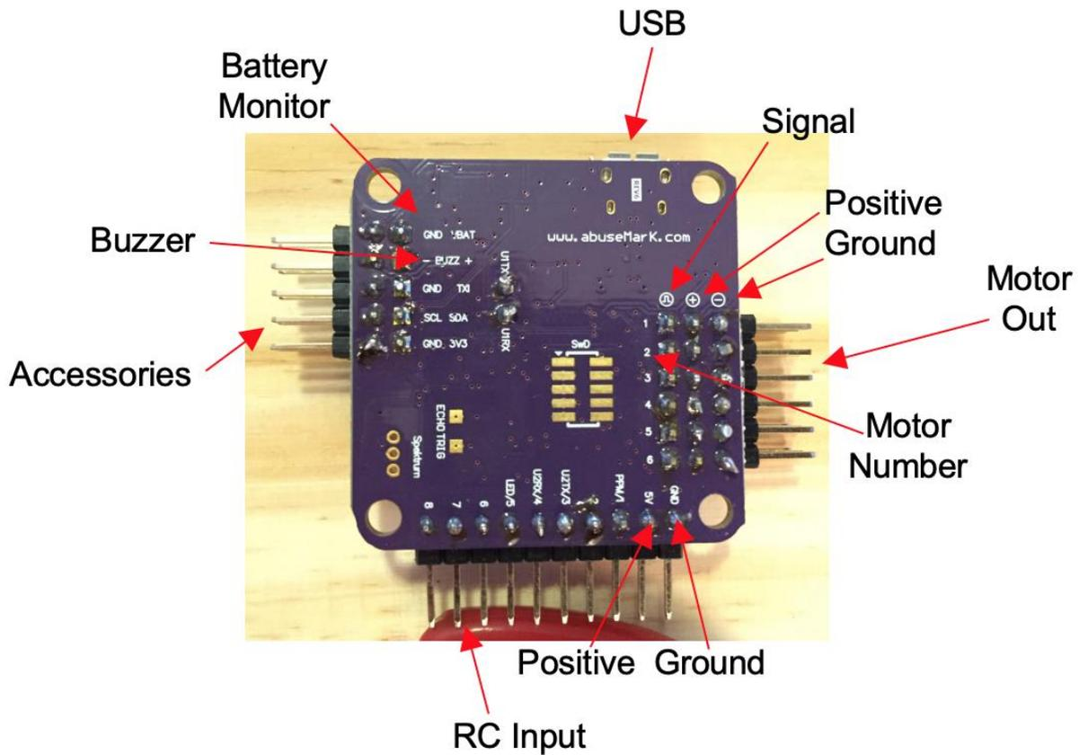
Figure 12: Flight Controller Setup
