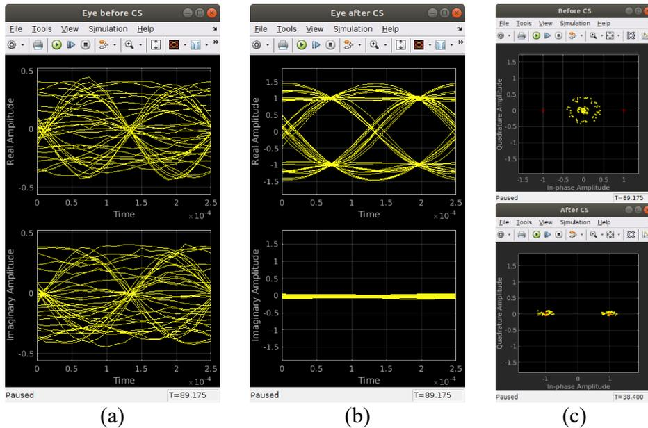
Figure 4: Example visualizations seen by students using the BPSK receiver. Panels (a) and (b) show eye diagrams before and after carrier synchronization, respectively. Panel (c) shows constellations diagrams before (top) and after (bottom) carrier synchronization.
