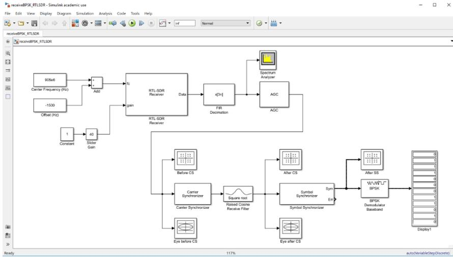
Figure 3: Simulink model for a BPSK receiver, including constellation and eye diagrams
