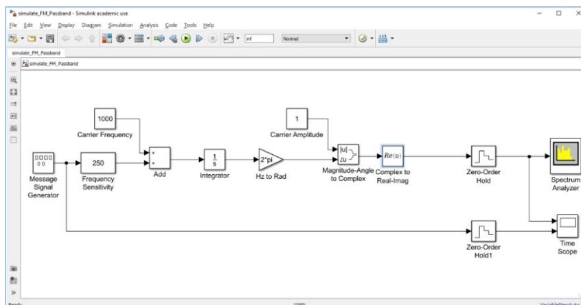
Figure 6: Simulink model for simulating passband FM waveforms
