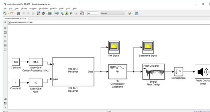
Figure 5: Simulink model for a receiving and listening to FM Radio (mono audio)
