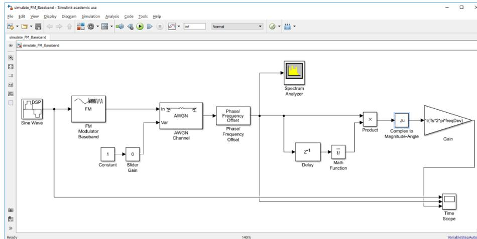
Figure 7: Simulink model for a simulating a baseband FM communication system.
