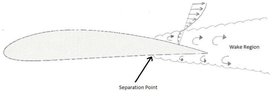
*Figure 2: Illustration of vector reversal and creation of wake zone*
