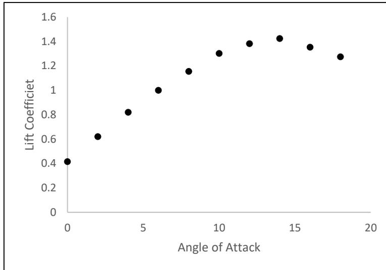
Figure 11: NACA 4414 baseline airfoil lift coefficient variation
