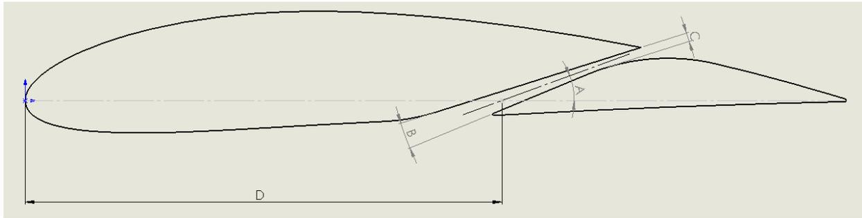
*Figure 13: 2-D view of slotted airfoil with geometric parameters. A: Slot angle to horizontal. B: Draft angle of slot. C: Slot width on suction side. D: Slot position in percent chord length*
