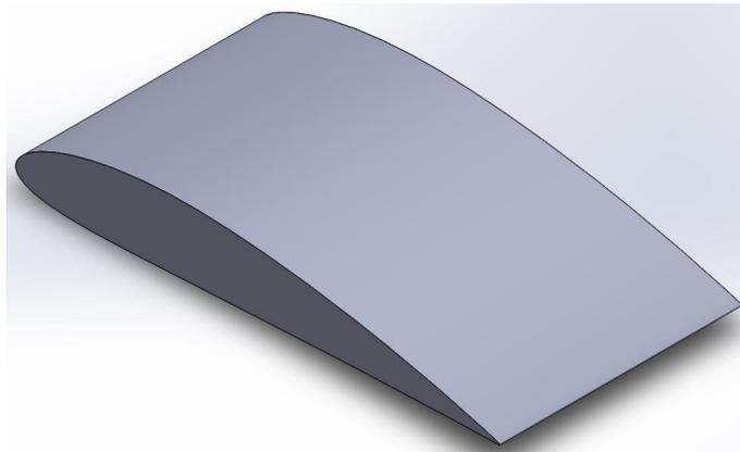
*Figure 9: 3-D view of NACA 4414 base airfoil*
