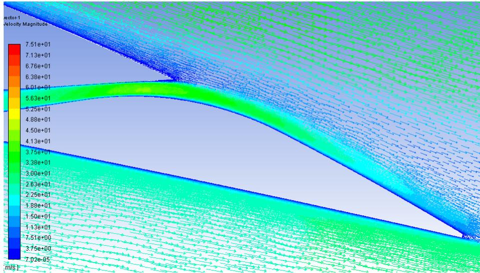
*Figure 17: Zoomed in view of velocity contours of 20-5-0.5-58 at  $14^\circ$*
