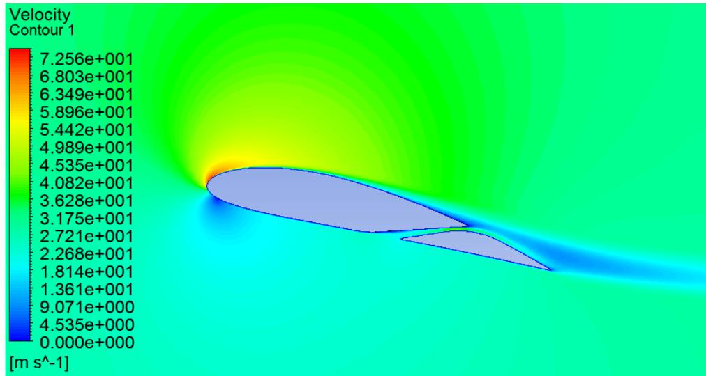
Figure 15: Velocity contour for NACA 4414 slot 20-5-0.5-58 at 14° angle of attack
