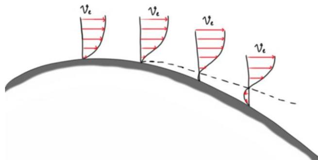
Figure 1: Velocity profile along airfoil
