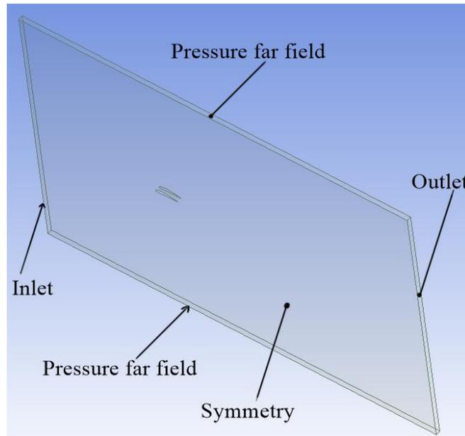
*Figure 10: Boundary conditions for 3-D case*
