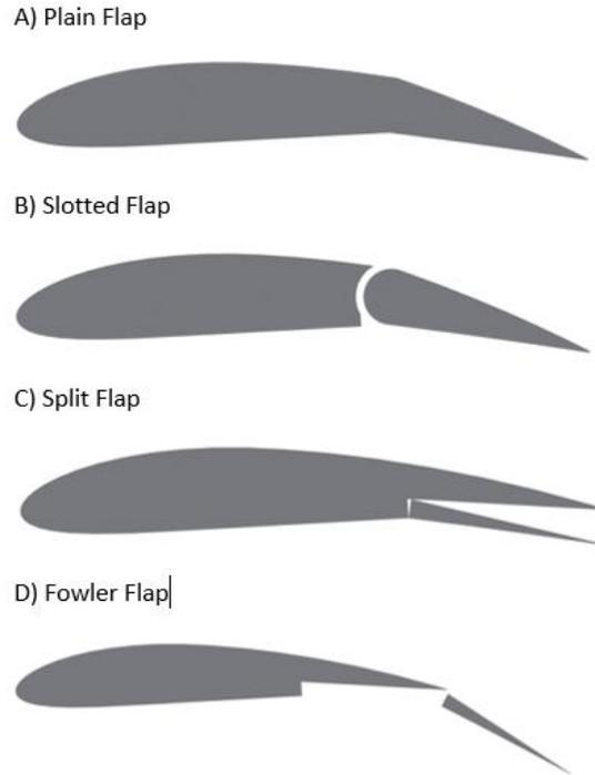
Figure 4: Trailing edge flap configurations.
