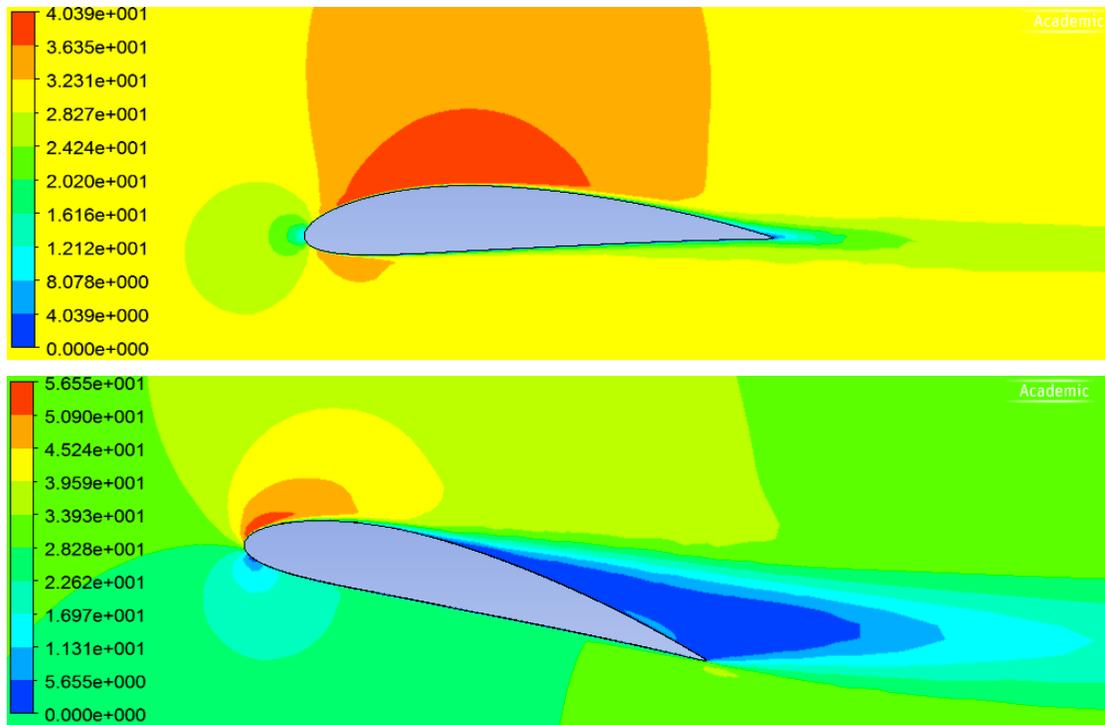
Figure 12: Close-up view of velocity contours for  $0^\circ$  (Top) and  $14^\circ$  (Bottom)
