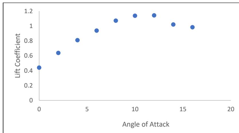
*Figure 3: Experimental results for lift coefficient with angle of attack for Clark-Y airfoil*
