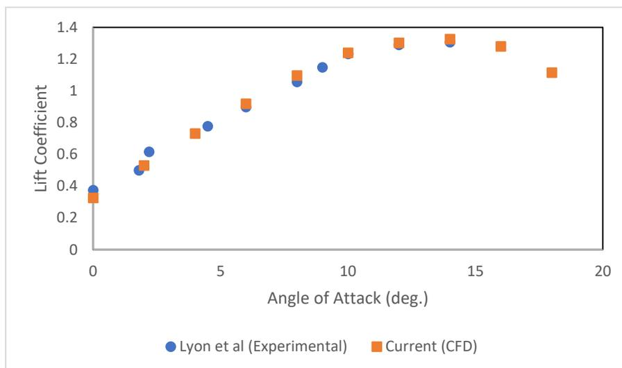
Figure 6: Experimental [13] and numerical comparison of lift coefficient for a Clark-Y airfoil
