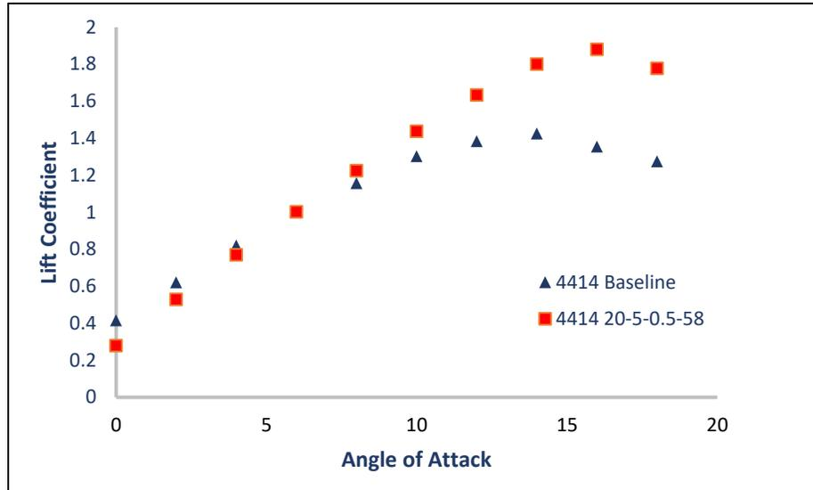
Figure 19: Comparison of lift data for NACA 4414 baseline and slot 20-5-0.5-58
