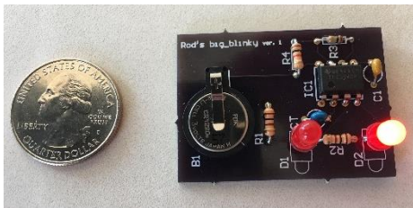
Figure 1—The completed, assembled, and working PCB design project: big_blinky
