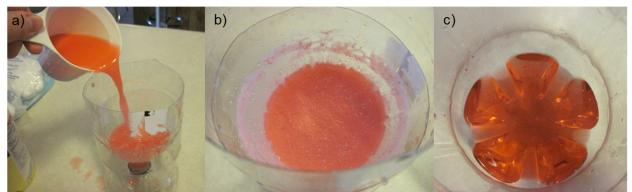
Figure 4: Mechanical filtration activity: a) pour the mixture of food coloring, water, and cornmeal over an inverted half soda bottle stoppered with a cotton ball and collect the filtrate in the other half of the bottle, b) the top half of the bottle has a residue of colored cornmeal above the cotton ball after the liquid drains completely, and c) the colored liquid passes through the cotton ball to be collected in the bottom half of the bottle.
