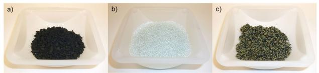
Figure 6: Materials for the chemical filtration activity: a) granulated activated carbon, b) 1 mm diameter glass beads, and c) contents of a water filter cartridge (for standard Brita pitcher models).
