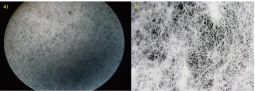
Figure 3: Light microscope images of a) paper coffee filter and b) cotton ball.
