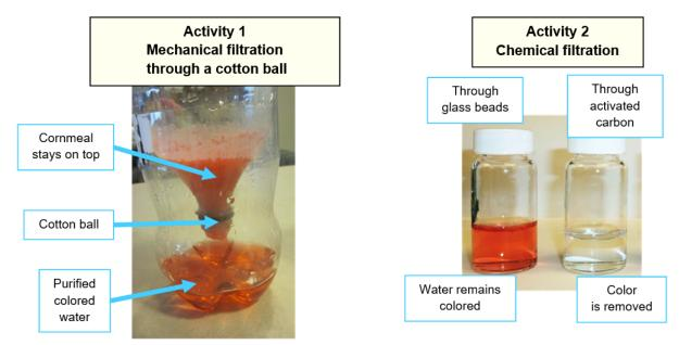
Figure 1: Experimental activities for demonstrating mechanical and chemical filtration.
