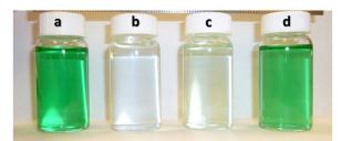
Figure 8: Chemical filtration results: a) original solution, which does not change after filtering through glass beads, b) 1 cup of original solution filtered through 1 cup of activated carbon,
