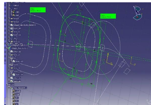
Figure 14. Port Cross Section from Four Arcs and Line Segments
