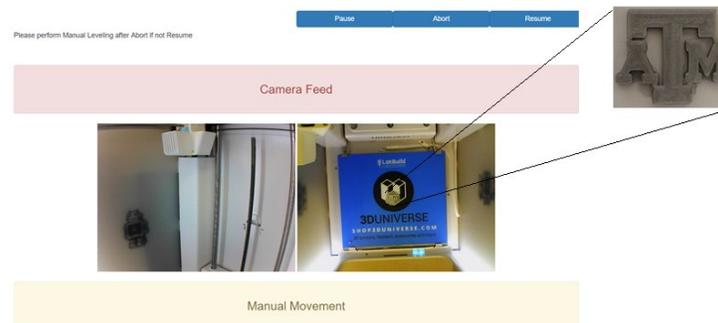
Figure 7. Uploading a file in Upload mode to print a logo.
