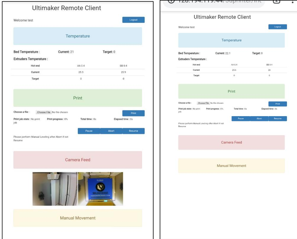
Figure 6. Client Main Web Page showing on the Mobile Device.
