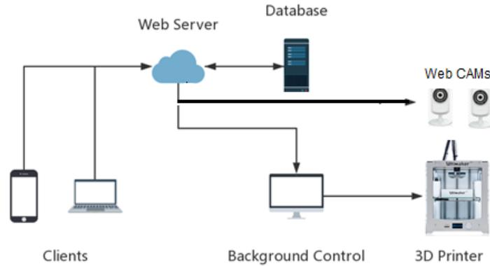
**Figure 1. System Components**
