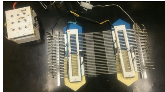
Figure 2: Image of the shuttle box apparatus. The controller is in the upper left corner.
