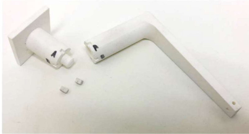
Figure 5: 3D Printed Door Handle Pass-Around Assembled and Disassembled, including Eraser Fragment Stress Elements
