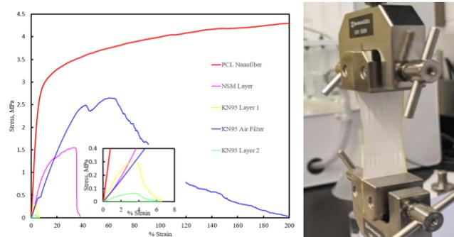
Figure 3. Stress-Strain diagram for a) PCL, NSM and KN95 filtration layers and b) tensile testing of PCL nanofiber
