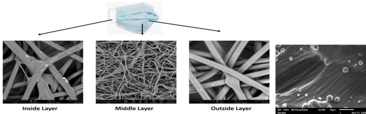
Figure 1. SEM Images of filtration layer of non-surgical mask and PCL nanofibers
