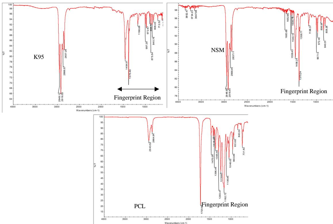
Figure 2. ATR results for Non-surgical Mask (NSM), K95 and Polycaprolactone (PCL) filtration layer
