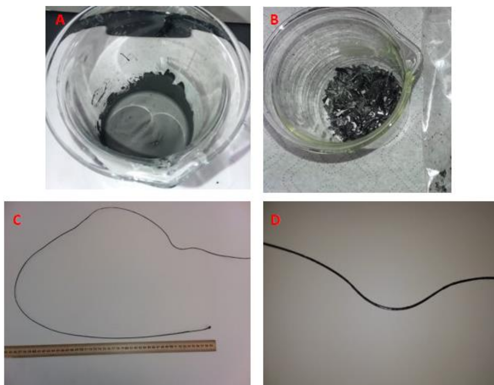
Figure 5: (A) Slurry for the graphite test 2-3. (B) PLA/Graphite pellets for test 2-3. (C) Obtained filaments (D) Close-up view of the obtained filament
