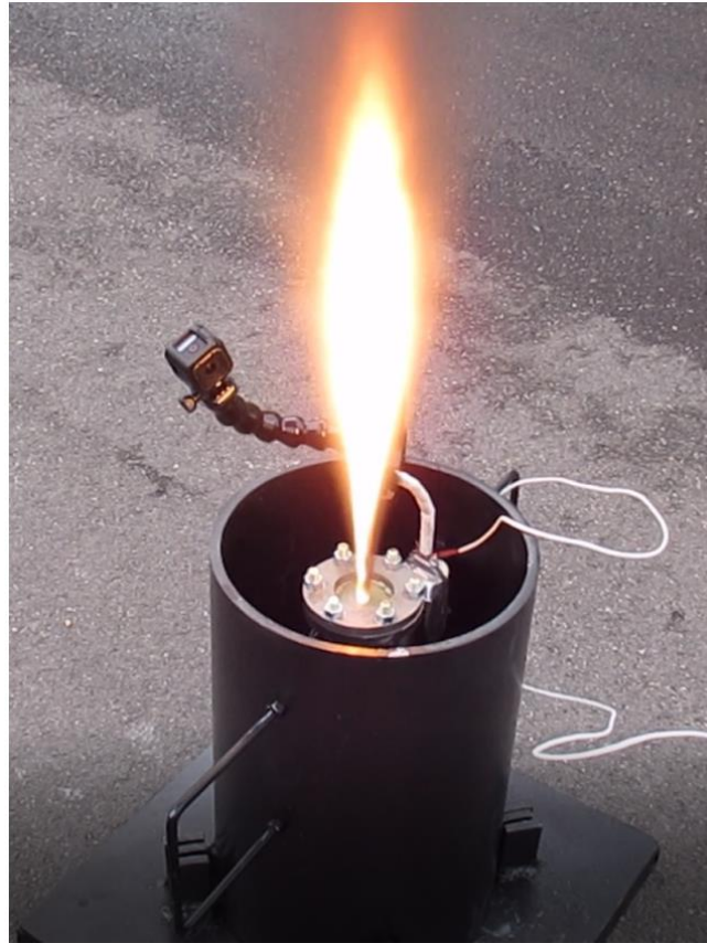
Figure 7 – CHRD Test Firing at Full Thrust (April 2021)
