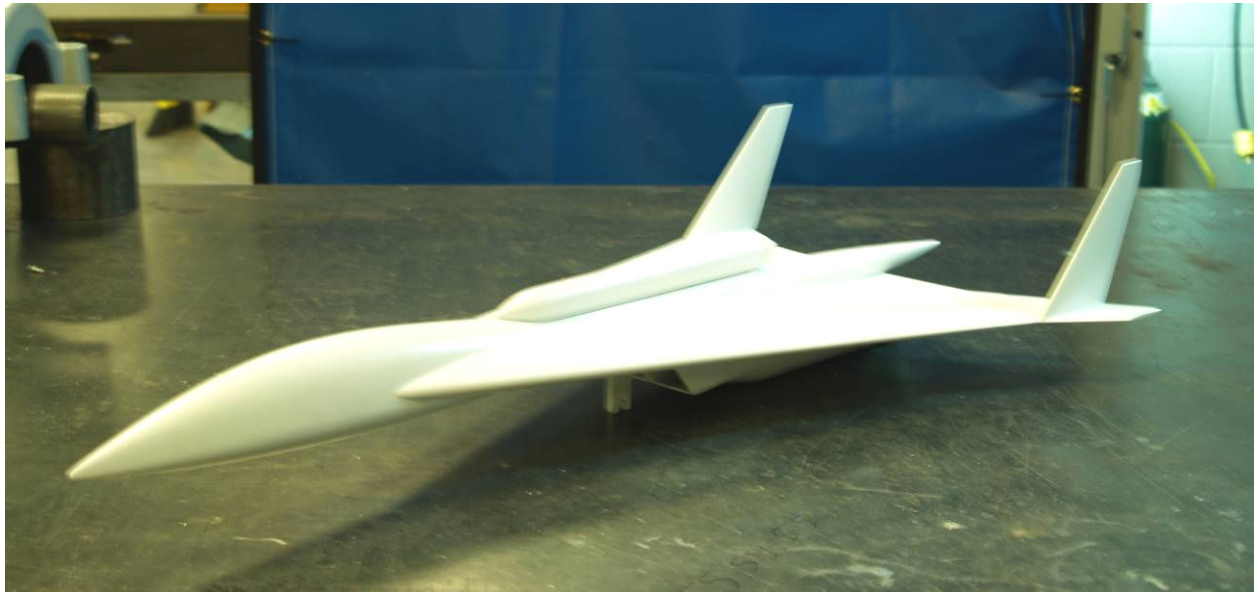
Figure 5: Wind Tunnel Model in Support of Wing Structural Design
