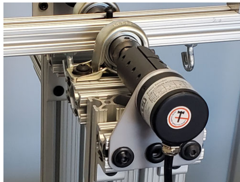
Figure 11. Rotary encoder on the shaft
