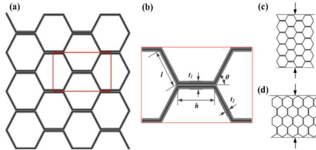
**Fig 3. Honeycomb infill pattern [5]**
