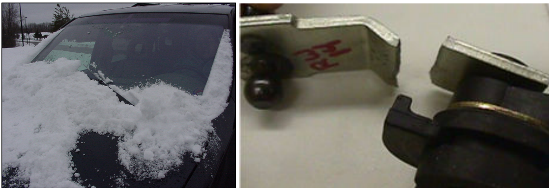
FIGURE 8 – WINDSHIELD WIPERS UNDER SNOW LOAD THAT BREAKS A ROCKER ARM
