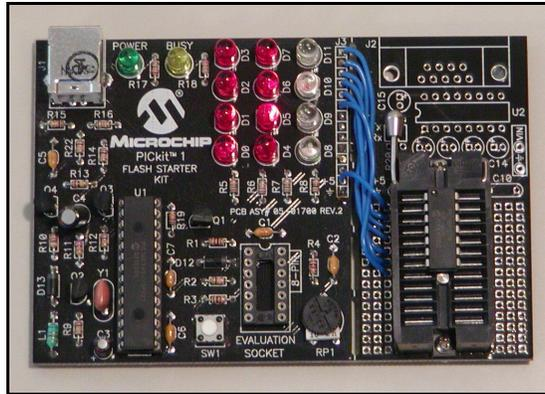
Figure 3. Modified PICKit1 Development Board
