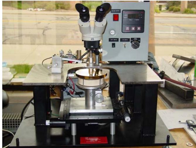
Figure 9. Photo of Wafer Testing Probe Station.
