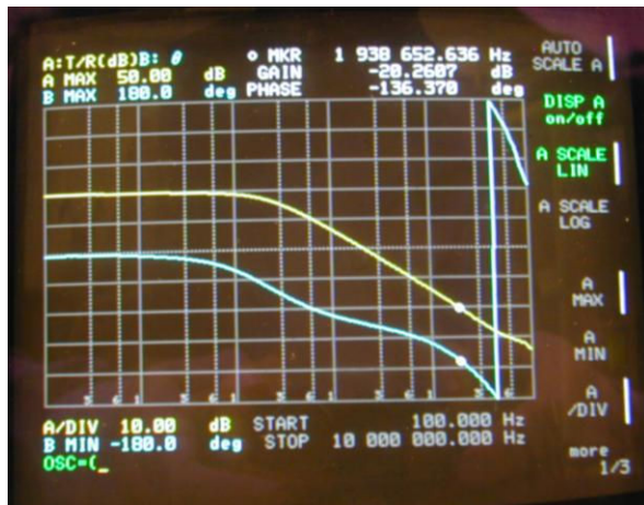
Figure 11. Frequency Response and Phase Margin
