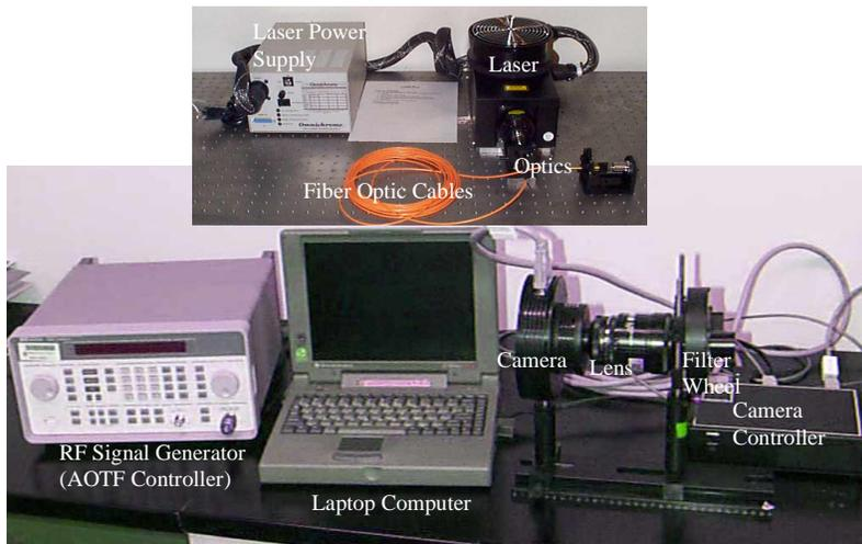
Figure 3. The Laser Induced Fluorescence Imaging System
