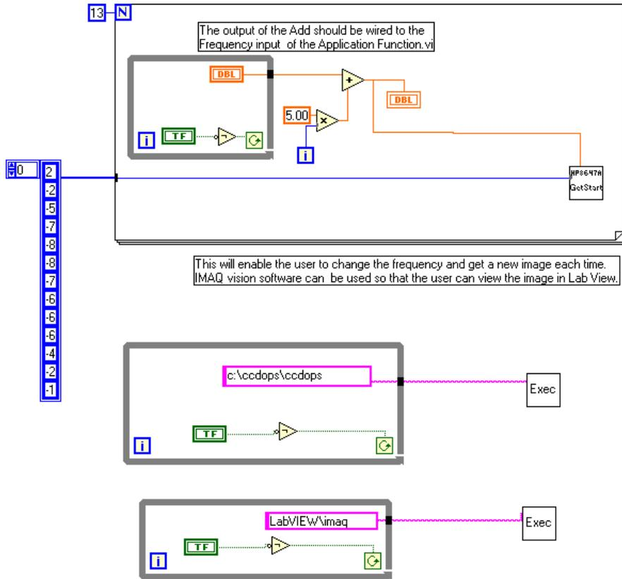
Figure 4. The VI Wiring Diagram for Controlling the AOTF.
