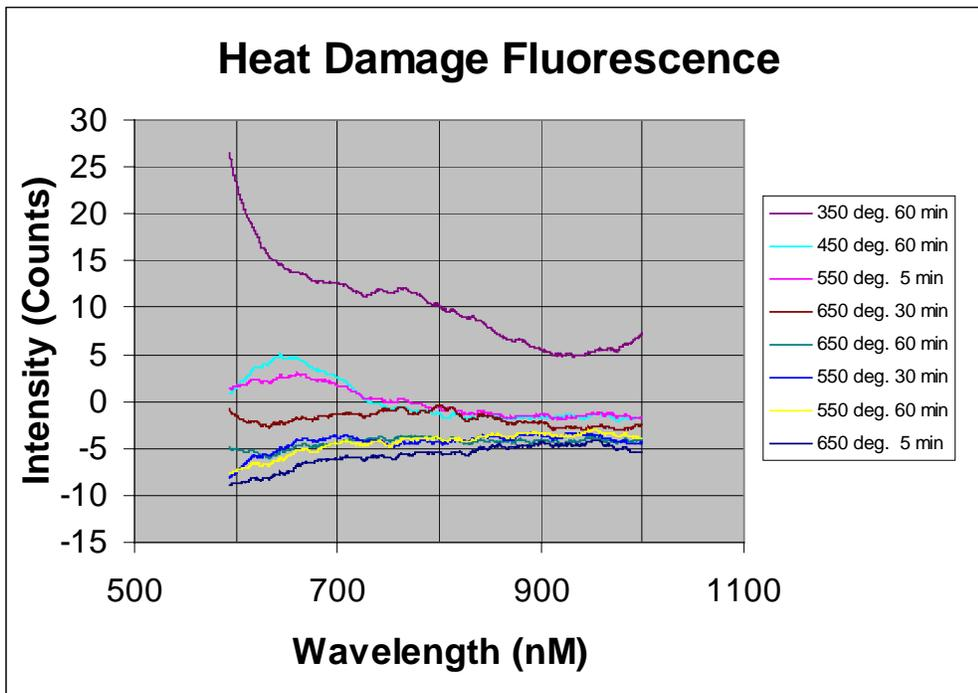
Figure 2. The Fluorescence Spectrum of Various Heat Damaged Coupons (sample-reference)
