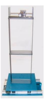
Figure 1. Bench-Scale Shake Table with Model Building and Active Mass Driver.
